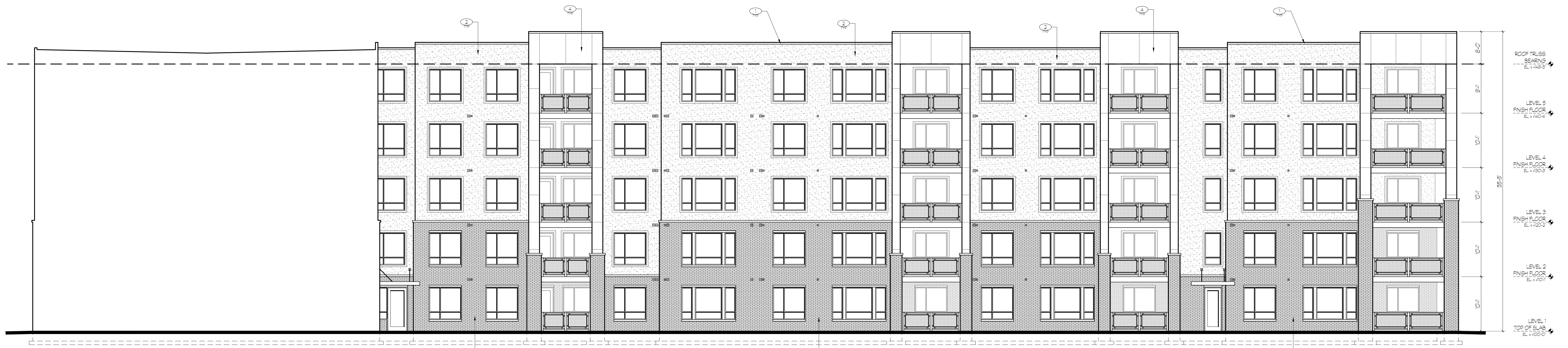
4 BUILDING ELEVATION EAST BUILDING C TSA SCALE: 1/16" = 1'-0" (30' x 42')
