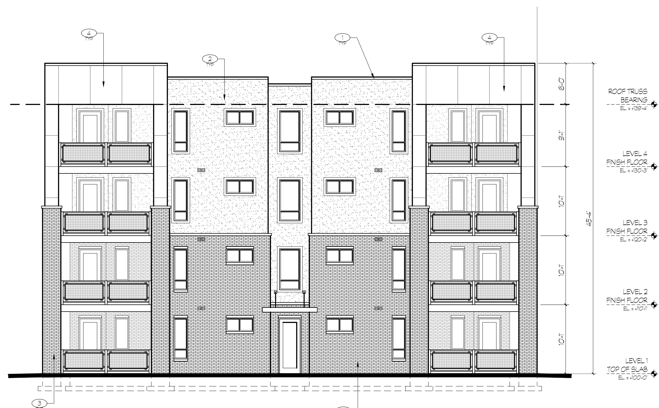
4 BUILDING ELEVATION SOUTH TSA SCALE: 1/16" = 1'-0" (30' x 42') BUILDING G
