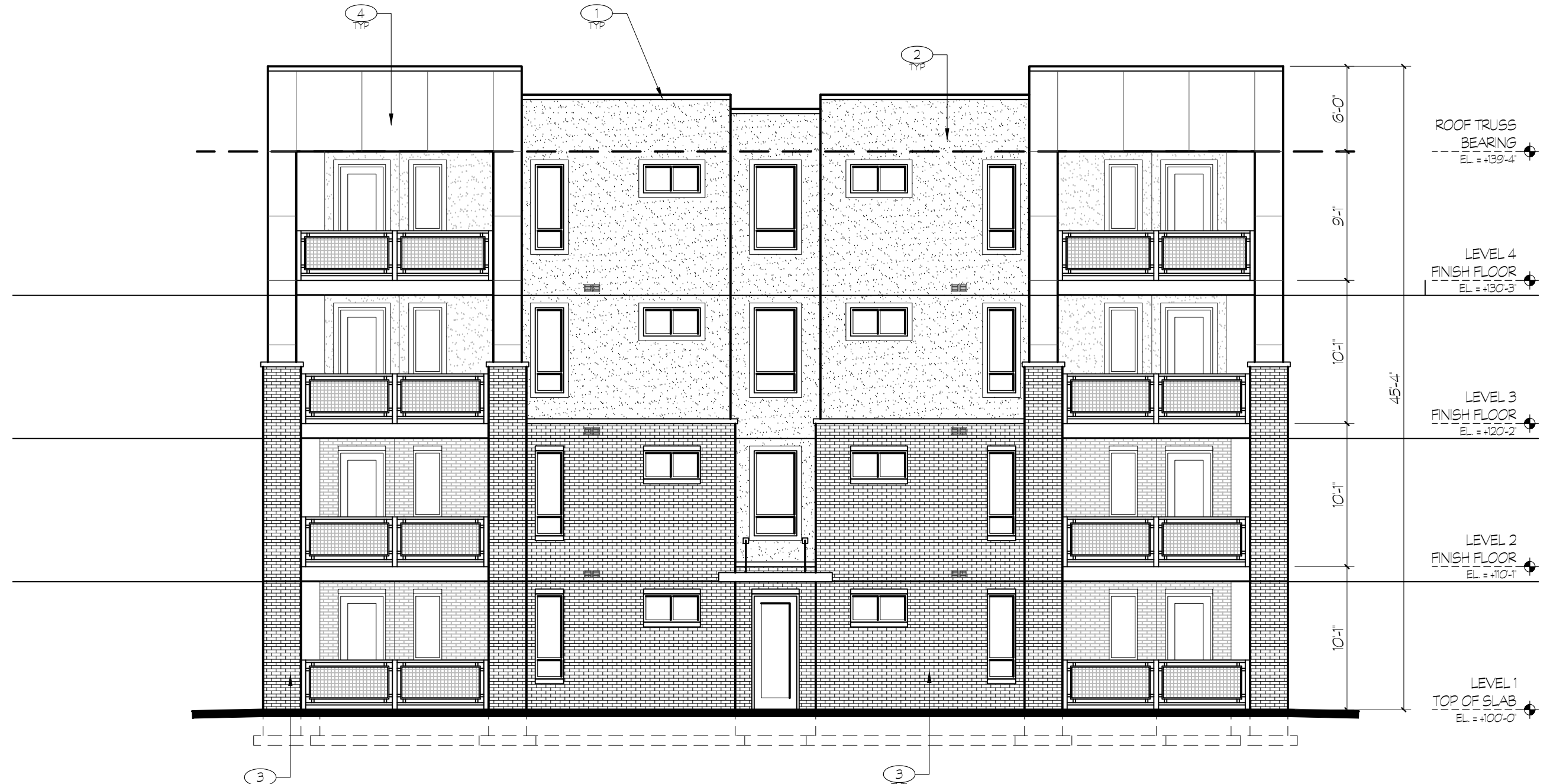
6 BUILDING ELEVATION WEST TSA SCALE: 1/8" = 1'-0" (30' x 42') BUILDING F
