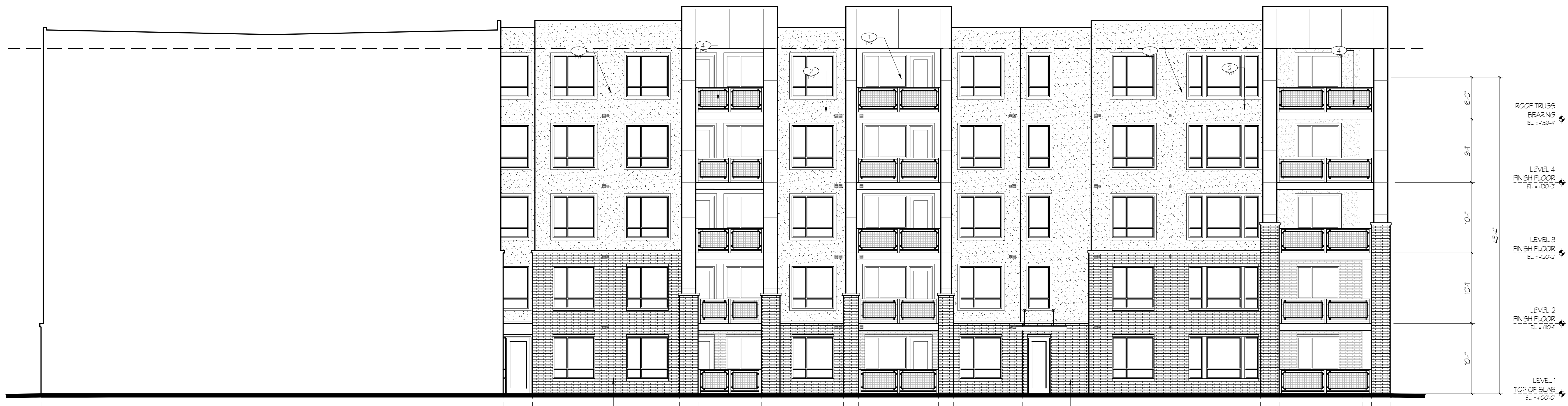
4 BUILDING ELEVATION SOUTH TSA SCALE: 1/8" = 1'-0" (30' x 42') BUILDING A
