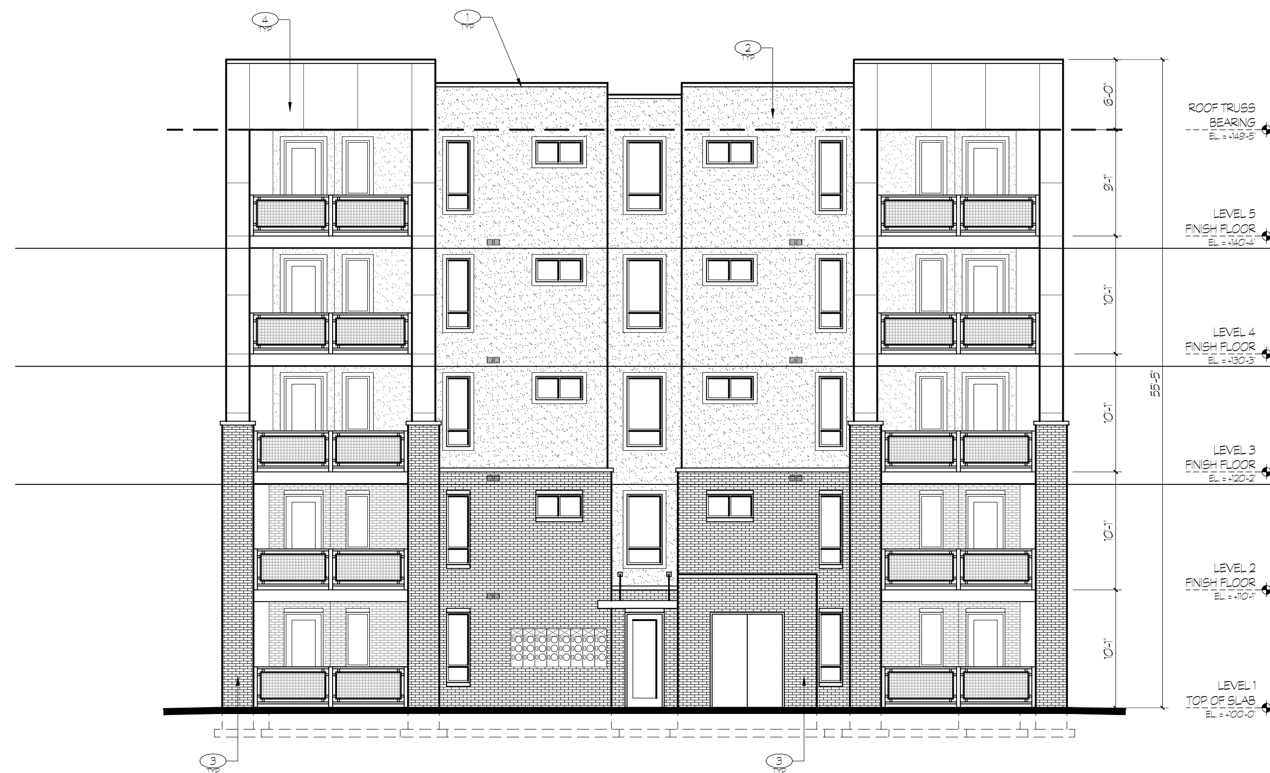
2 BUILDING ELEVATION NORTH BUILDING E TSA SCALE: 1/8" = 1'-0" (30' x 42')
