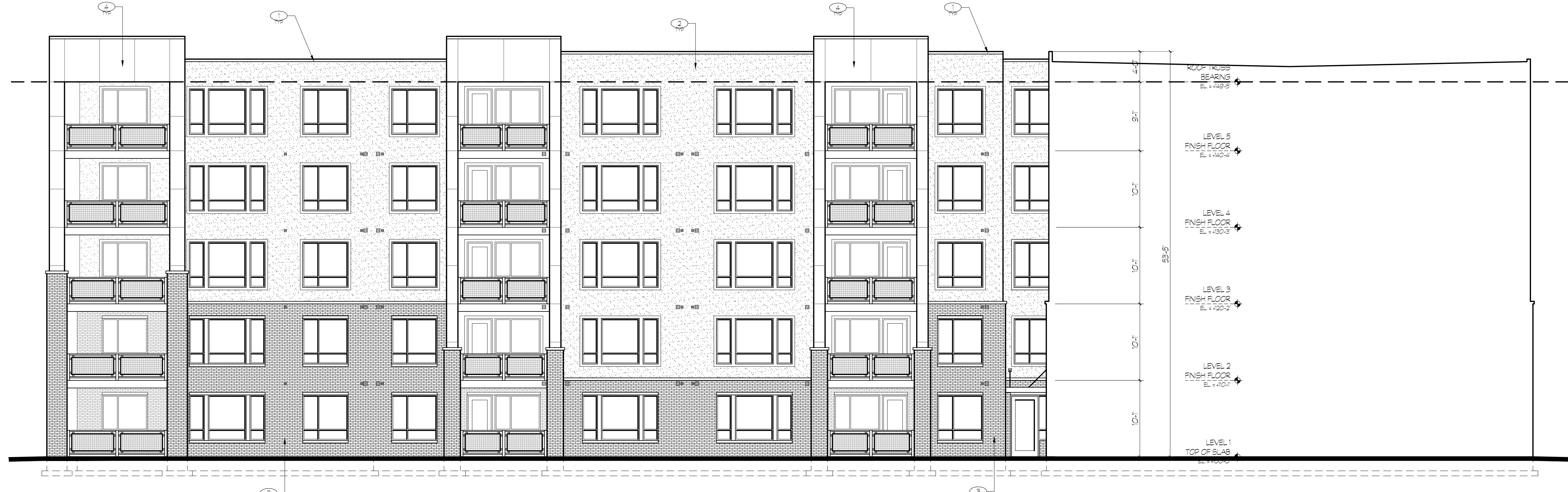
5 BUILDING ELEVATION WEST TSA SCALE: 1/16" = 1'-0" (30' x 42') BUILDING D
